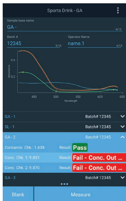
Figure 5: GENESYS Smart QC "Sports Drink – GA" method results for GA-2: 10% v/v GA.
