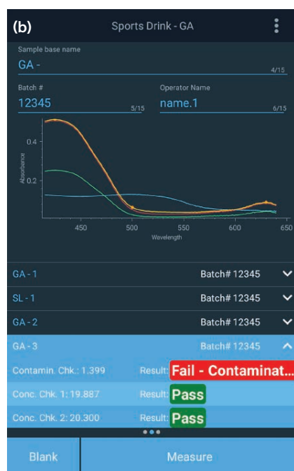
Figure 6: (a) Images of GA samples with (left) and without (right) SL contamination. (b) GENESYS Smart QC results for GA-3: 20% v/v GA spiked with SL (SL concentration = 2.0 %).
