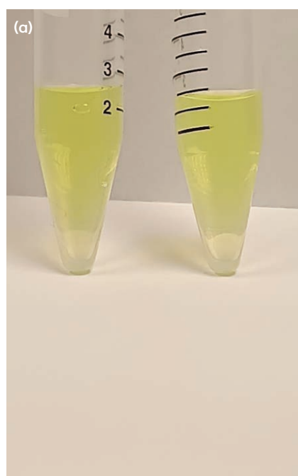
Figure 6: (a) Images of GA samples with (left) and without (right) SL contamination. (b) GENESYS Smart QC results for GA-3: 20% v/v GA spiked with SL (SL concentration = 2.0 %).
