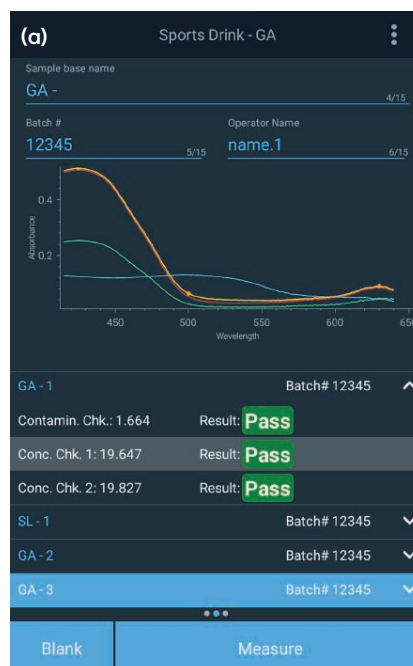
Figure 4: GENESYS Smart QC "Sports Drink – GA" method results for (a) GA-1: 20% v/v GA standard and (b) SL-1: 20% v/v SL standard.
